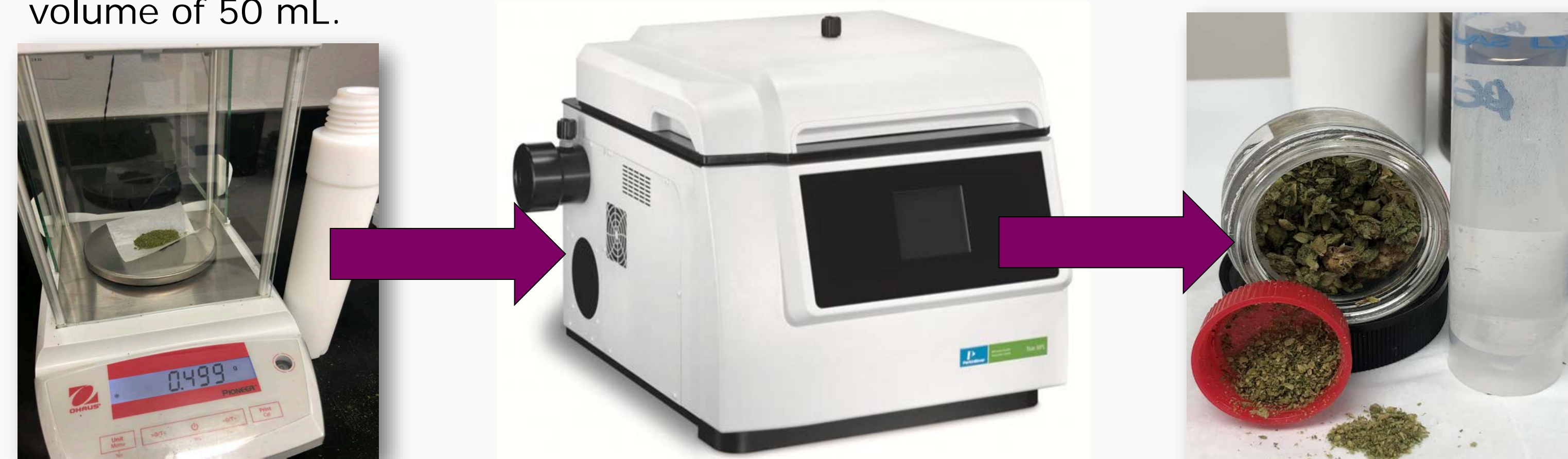
Figures 1-3. Workflow for sample preparation, from weighing to digestion, and final clear digestate.
